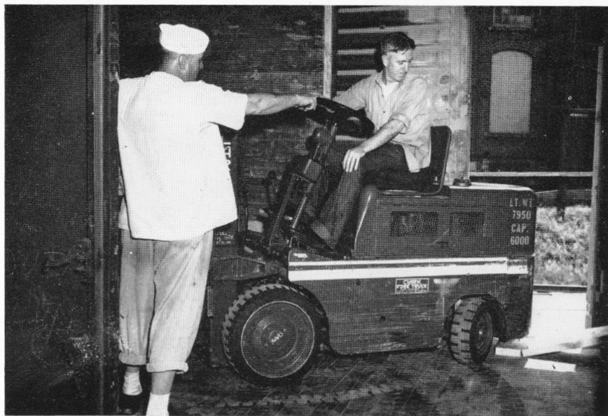
Frank McFarlin (with back to near-side open door) and James Cunningham (driver) of the North Mill demonstrate one method of preventing a fork lift truck from accidentally rolling out of an open freight car door.
